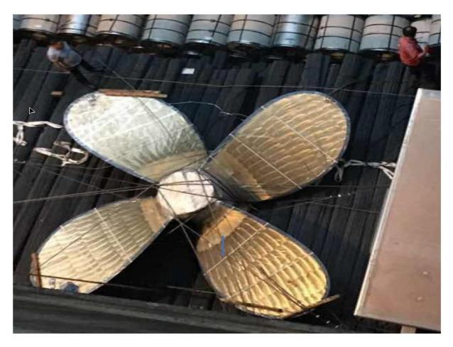
PROPELLER 4 Blades, Pitch 3810 mm, Weight: 13 Ton Ni-Al Bronze with LR Class
